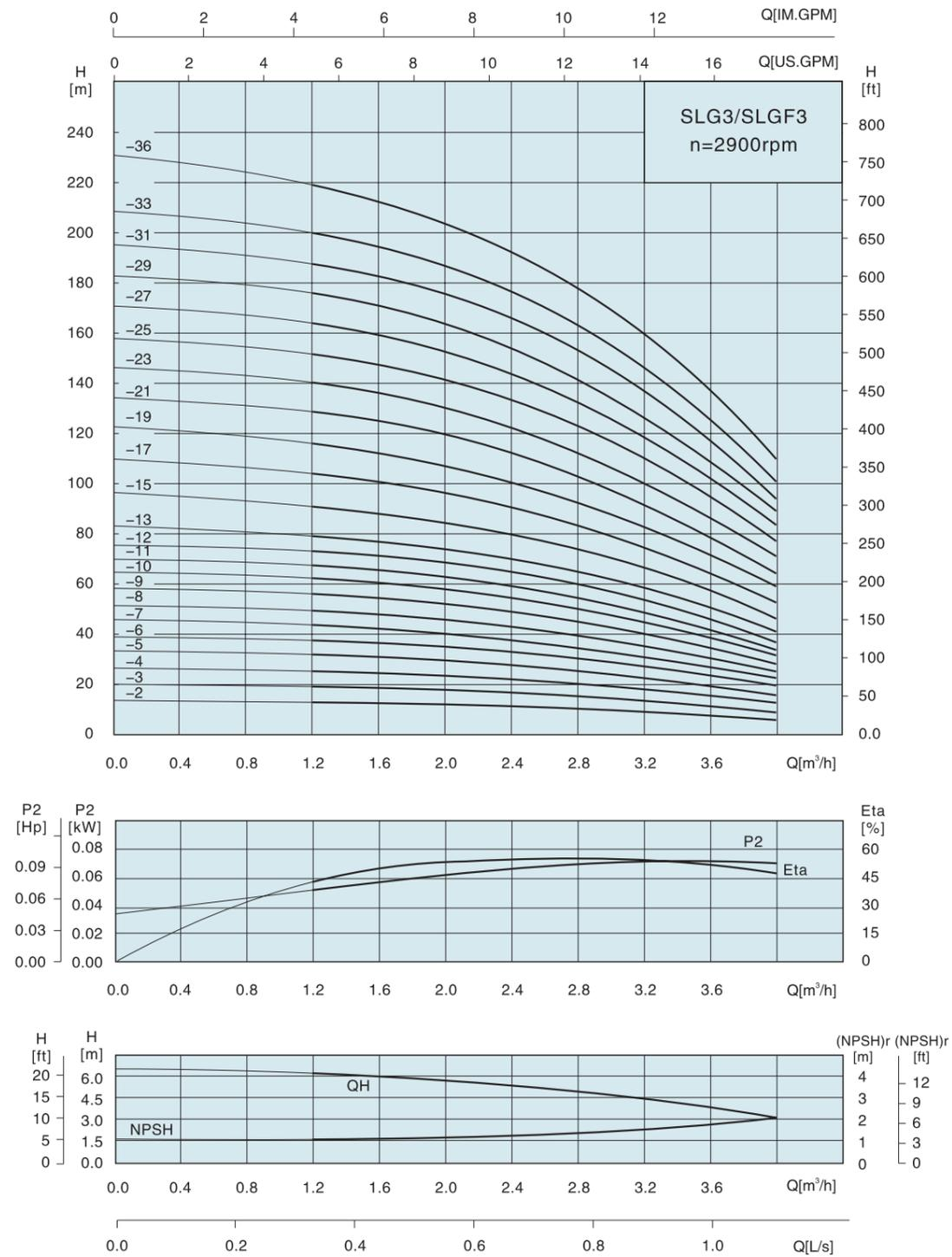
性能表及安装尺寸图表 Performance table and installation dimension
