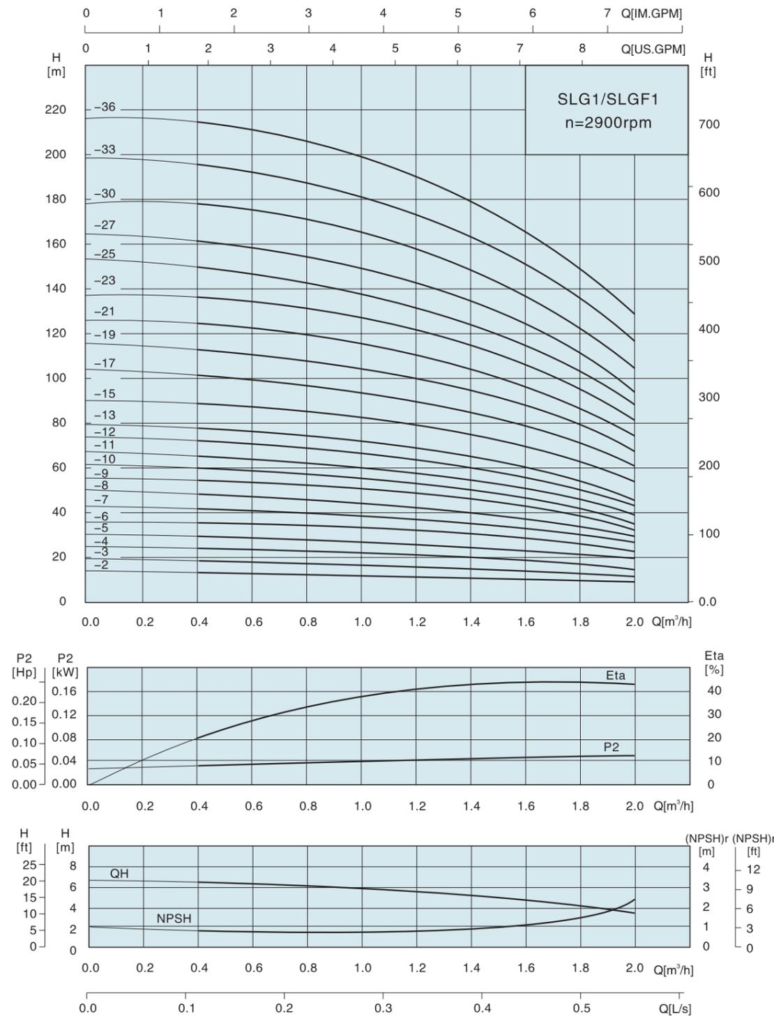
性能表及安装尺寸图表 Performance table and installation dimension
